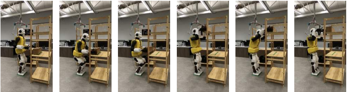
Fig. 4: Whole-body Controller Method Motion Sequence
